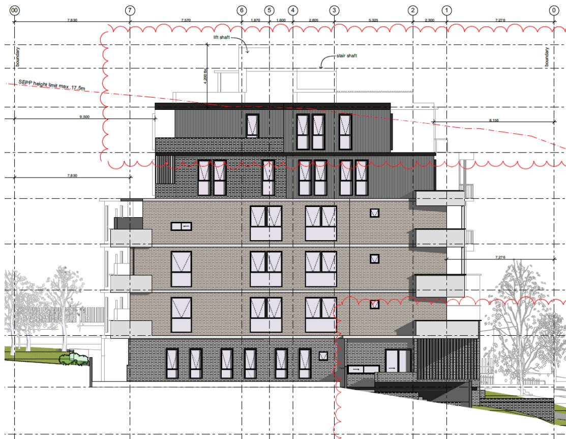
Figure 22: South Elevation Showing Southern Edge Non-Compliance
